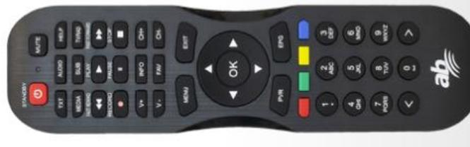
**The remote control is ergonomically designed, visually attractive, but has a slightly unexpected key layout with the number keys at the lower part**
